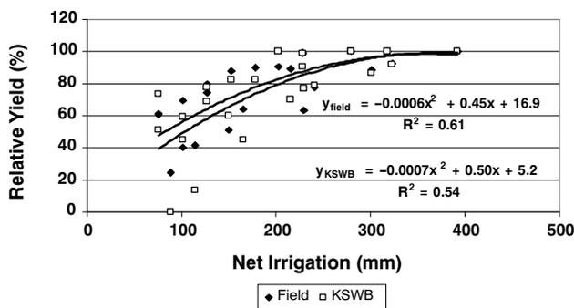
Figure 7. Relative yield over years vs. net irrigation from field data and the KSWB.
