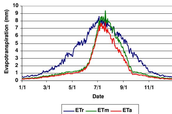
Figure 2. Example of reference ET ( $ET_r$ ), maximum ET ( $ET_m$ ), and actual ET ( $ET_a$ ) from an execution of the Kansas water budget.
