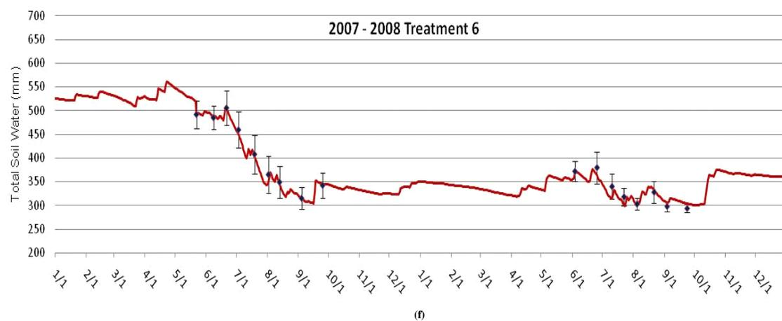
Figure 3 (con't). Total soil water for irrigation treatments 1-6 from 2005-2008 (solid line from KSWB and discrete points from field measurements with  $\pm 1$  standard deviation error bars).
